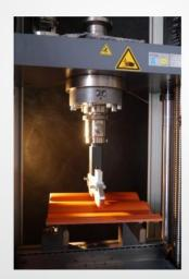
Transverse Breaking Strength Test
